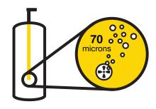
First, the Multi-Rotors located within the **system turn water into droplets of 40-80 micron** size by mixing it with air in a pre-set proportion.
