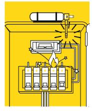
**Stage 1:** A fire sparked by a short circuit causes the pressure inside the Mini's glass bulb to increase.
