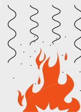
Mist turns into steam, covering the flames and lowering the temperature
