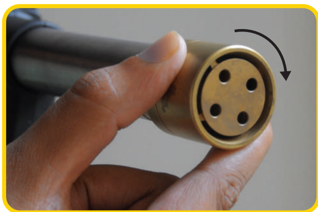
Fine spray to fight close range Class A fires such as fires in wood, paper and cloth, and electrically started fires.
