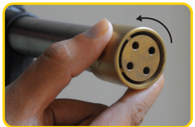
Wide throw to combat Class B (oil, petrol, paint) fires.
